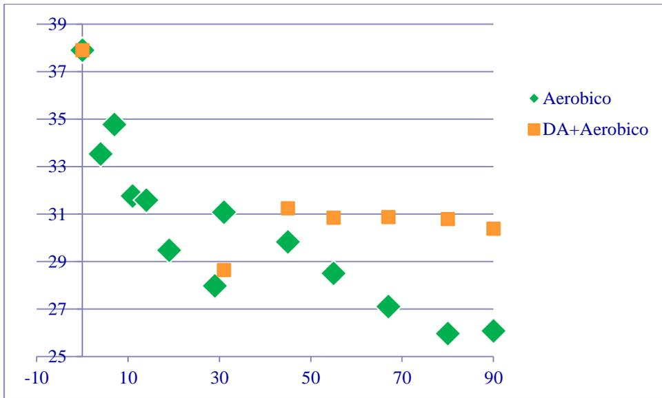
**Fig. 3.** Evolution of the organic carbon concentration of the OFMSW for aerobic and AD+aerobic treatment.
